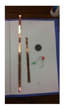
Grab one long and one short piece of copper tape, two LEDs with colors of your choice, and one button cell battery.
