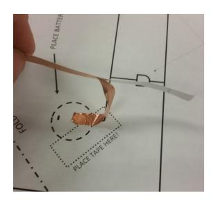
Take the short piece of copper tape, peel back about one inch of backing, and attach the tape to the solid line that starts on the battery spot.
