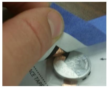
Make sure that when you fold the switch flap, the copper tape on the flap makes contact with the metal on the top of the battery. If it doesn't, adjust your fold.
