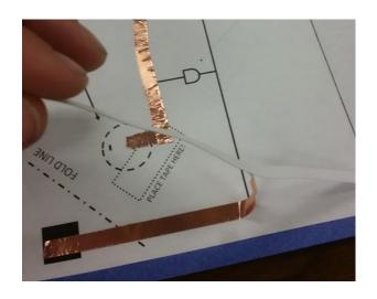
Take the long piece of copper tape and attach one end to the black square. Place the tape along the solid line and remember to peel the backing off as you go along!
