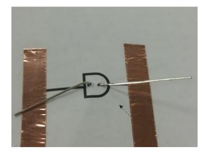
Bend the leads of the LED so they cross the copper tape, as shown on the left.
