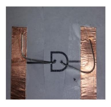
If the lights flicker or do not turn on, try folding the leads of the LEDs so they run along the copper tape as shown in the picture.
