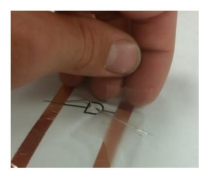
Secure the leads of the LED to the copper tape with clear scotch tape. Make sure to push the tape on hard so that a solid connection is made between the copper tape and the LED leads.
