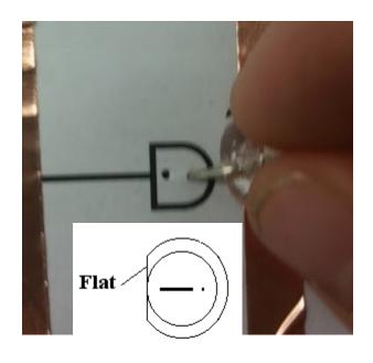
Using a push pin, poke two holes side-byside through the paper on the LED spots.
