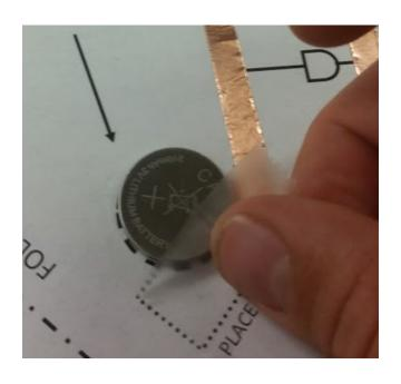
After Both pieces of copper tape are placed, use a piece of clear scotch tape to secure the batter in the designated spot. Make sure that the tape only covers a small edge of the battery and that the "+" side of the battery faces up.
