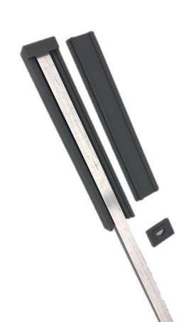
1) Prepare the mold for the inner layer and the aluminum-rod core
