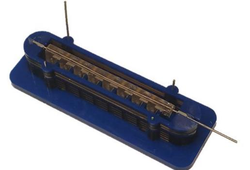
3) Once the core has cured, set it in the actuator mold and use the mold to cast the actuator out of an elastomer
