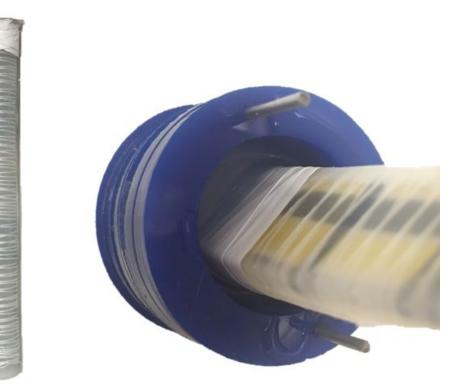
5) Once cured, demold the actuator, wrap the end in Teflon tape, and cap the end with an elastomer
