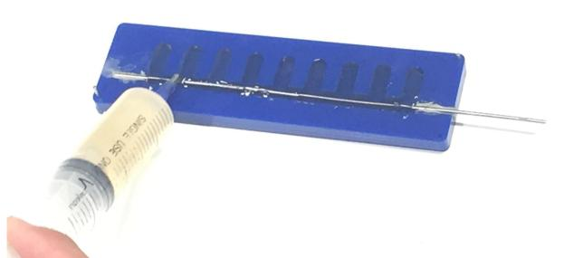
2) Cast the core out of a meltable material (e.g. glycerol-gelatine mixture)
