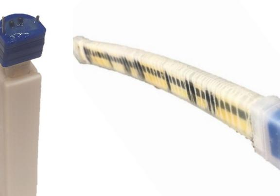
7) To finish, attach the "fingernail" connector to the other end of the actuator so that the "fingernail" pieces can be attached
