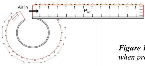
Figure 1. The motion of a pneumatic actuator when pressurized with air (Polygerinos et al.).
