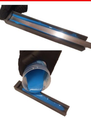
2) Cast the inner layer out of an elastomer
