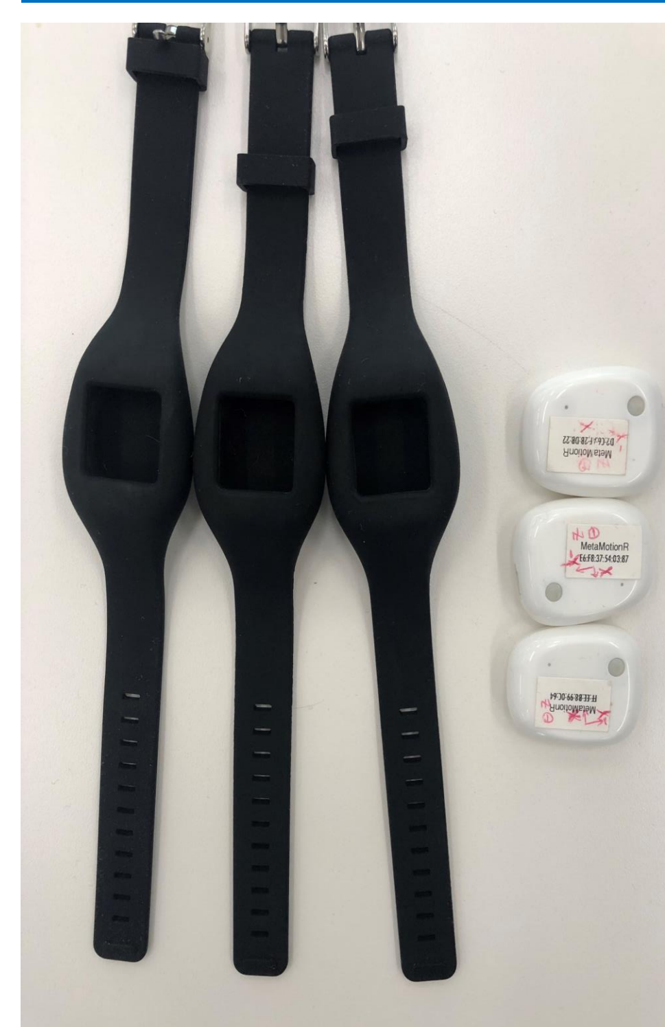
Figure 2: MetaMotionR Accelerometer Sensors Used for lab-experimental exercises and recordings
