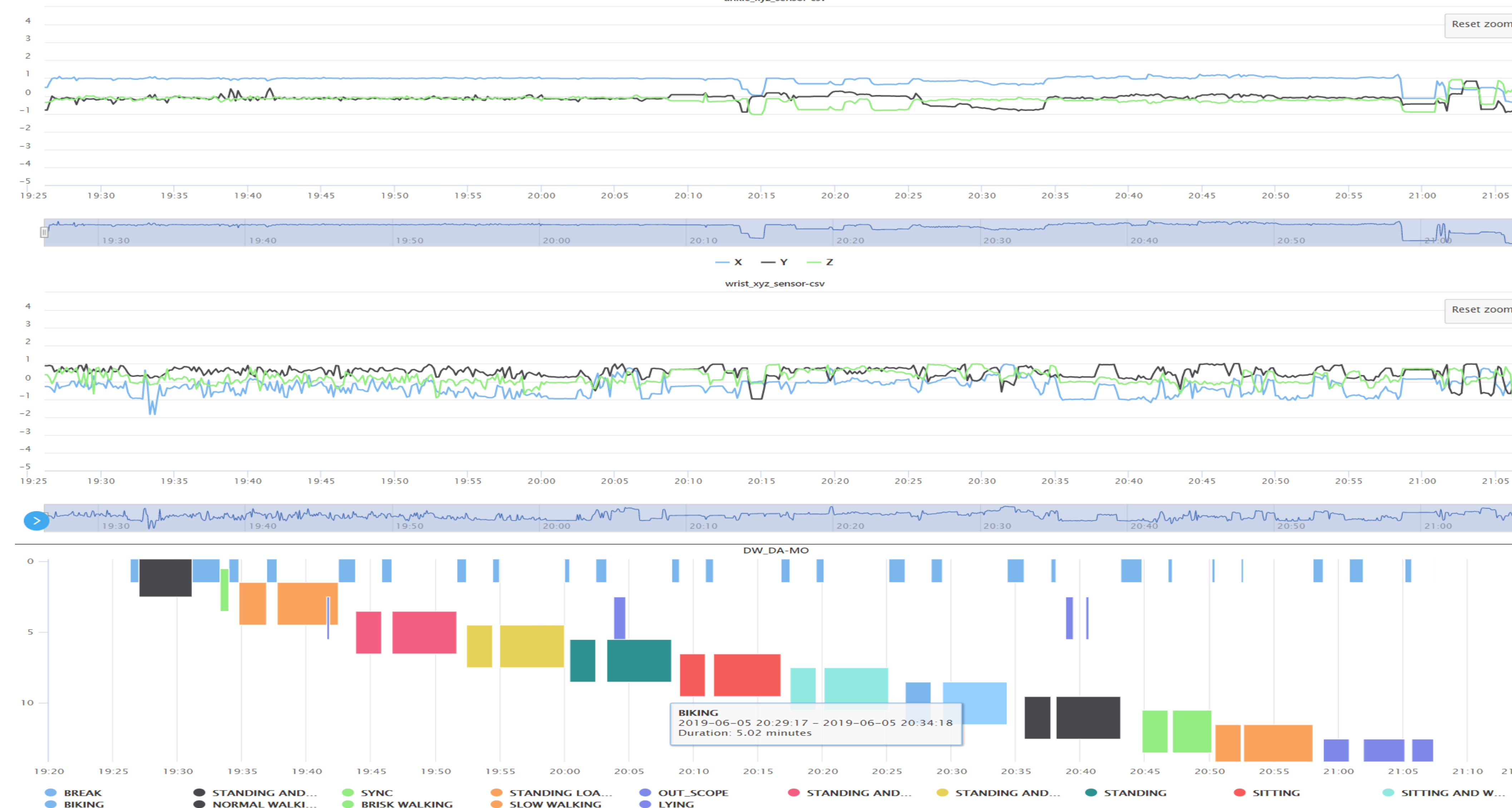
Figure 6: Ankle Sensor | Wrist Sensor | Activity Annotation Graph (Activities that were performed with the corresponding time and data above)
