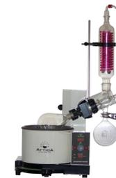
Figure 6. Rotary evaporator used to evaporate chloroform from the lipid film. <https://www.kisspng.com/png-distillation-rotary-evaporator-laboratory-evaporat-5834303/preview.html>
