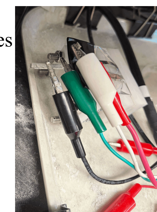
Cell with 20 mg graphite during cycling
