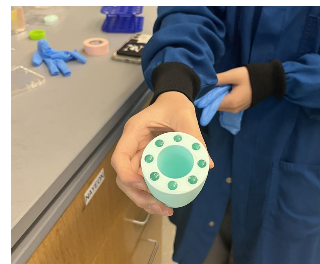
Figure 4. 3D Printed Mold with PDMS inside
