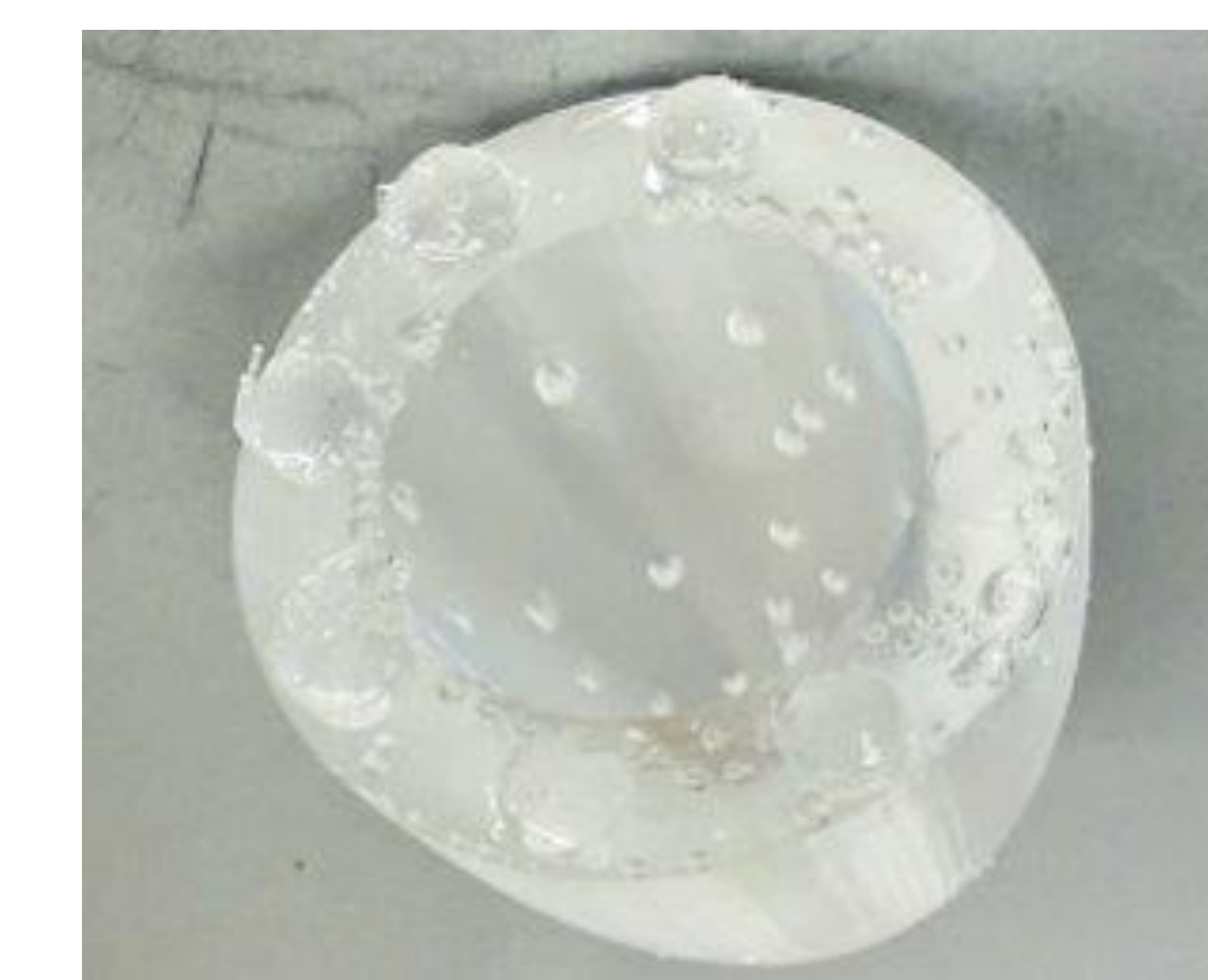
Figure 5. Completed Polymer Ventricle Model
