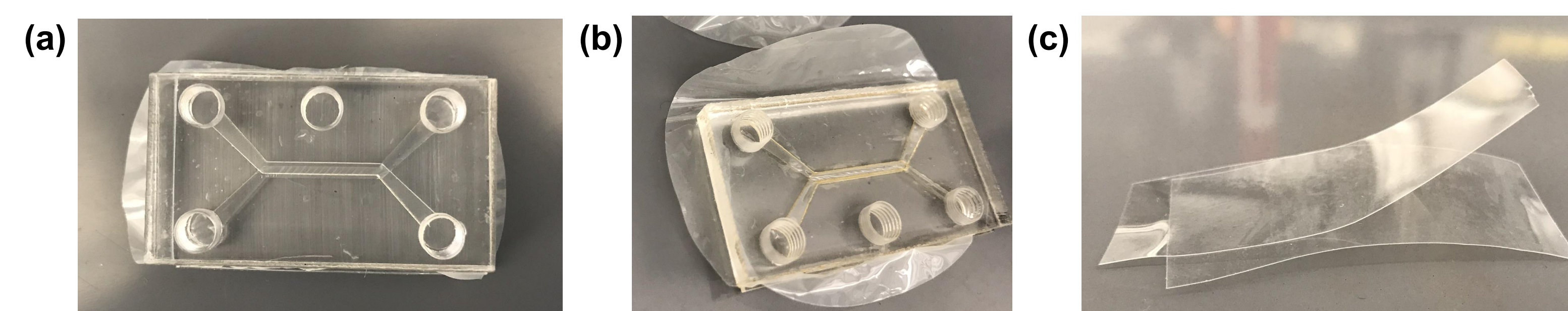
FIGURE 4. (a) Polymethylmethacrylate (PMMA) chip was fabricated at 145°C for 10 minutes following surface treatments. PMMA chips had decent optical clarity but were prone to air bubbles. (b) Polycarbonate (PC) chip was fabricated at 160°C for 10 minutes following surface treatments. PC chips had similar optical clarity but were less prone to air bubbles. (c) Attempted thermal bonding of polyethylene terephthalate (PET) was unsuccessful.
