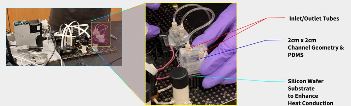
Performance of a Microfluidic Device in a System for Detecting the Presence of COVID-19 RNA
