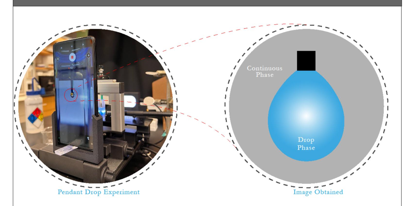
The pendant drop method is a widely utilized technique to measure the surface tension of liquids. This method involves analyzing the shape of a drop hanging from a blunt ended needle, on the verge of detachment. In our experiment, we employed Polyethylene Glycol Diacrylate (PEGDA) in water as the drop phase and mineral oil as the continuous phase. Due to their immiscibility, these phases do not form a homogeneous mixture, allowing us to measure the surface tension.
