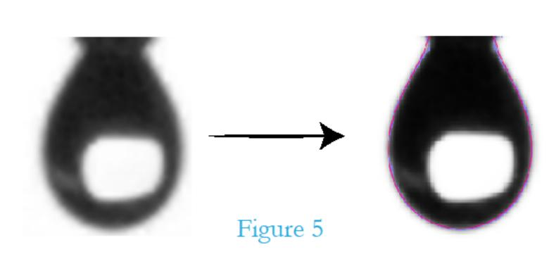
We use software called Open Drop to sharpen the images of each drop. Figure 5 shows a drop image before and after using Open Drop. Ten analyses are conducted for each solution, with subsequent calculation of an average value. Figure 6 shows the average surface tension as a function of PEGDA concentration. Surface tension decreases because the polymer can adsorb to the interface.
