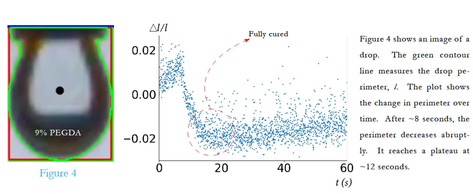
This plateau, ~2% smaller than the original perimater, indicates the drop is fully cured. The light is placed 37.33 mm from the needle, and the minimum dosage is 133.5 mj/cm^2.
