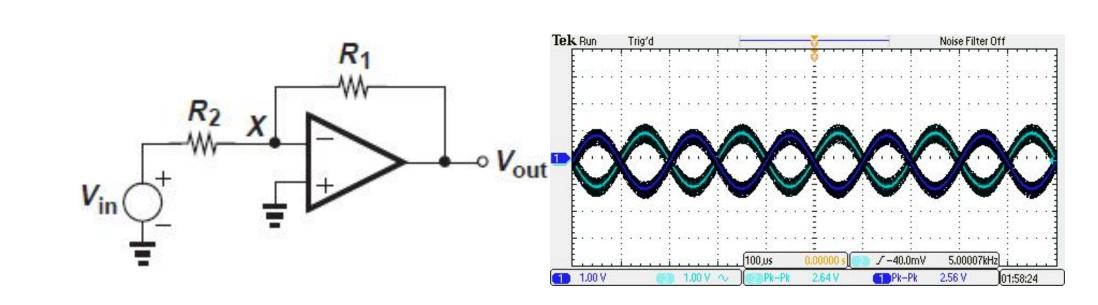
Op - Amp placed in feedback loop with R2 =  $R1 = 10 \text{ K}\Omega$
